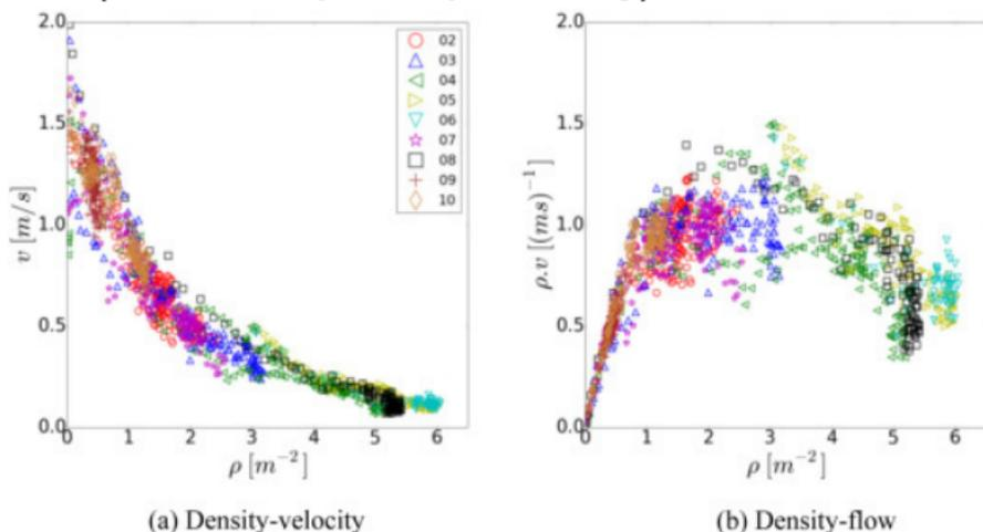
**Figure 1:** Fundamental diagrams for pedestrian traffic flow in controlled experiments Wang et al 2019
